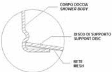
An alternative system to welding is caulking, the body of the shower is folded over the mesh to lock it in place.
